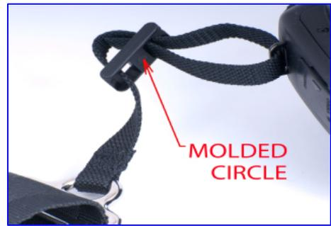
4. Continue threading the free end back through the sliplock so that it looks like the photo at right. There should be at least 1/2" of free end extending beyond the 3/8" slip-lock. When adjusting the OP Tail, it helps to keep the webbing loose as shown in the photo.
